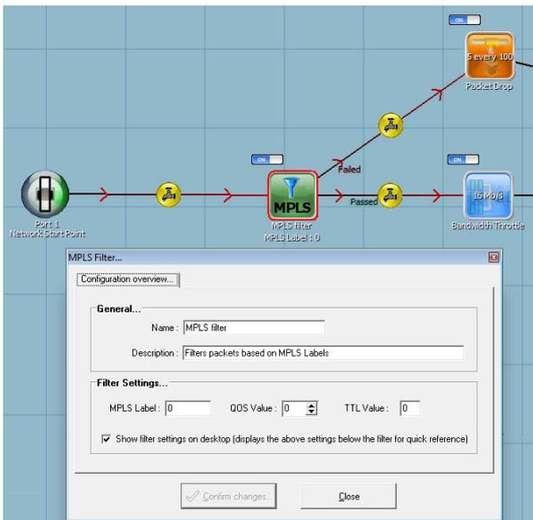
By emulating a network, the size, router specifications and topology can all be controlled through the use of a 'Drag and Drop' User Interface. This allows for more flexible and larger scale testing than in a real network and costs are significantly reduced since no expensive network devices are needed. JAR:Emulate is beneficial for testing in real-time the conditions found on MPLS networks.
